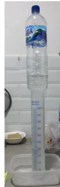
Figure 3. Equipment Built to Measure Reynolds Number
