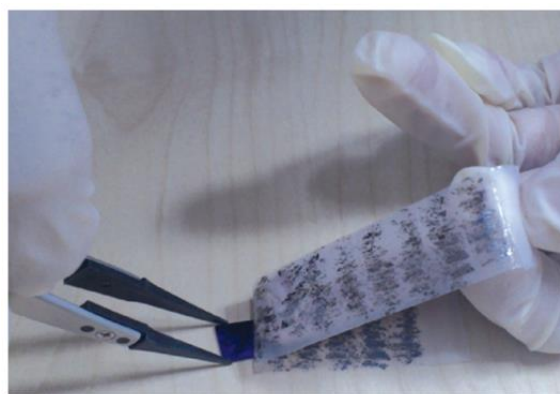
Figure 5. The technique for synthesizing graphene using the "Scotch tape" method was initially documented in 2004 by Novoselov and Geim [Mbayachi, 2021]
