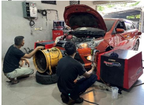
Figure 3.4 : Hub-Chassis Dynamometer Test Setup
