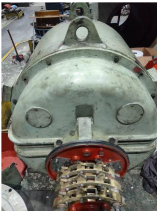
Figure 2. 1: Photograph of 3p-SR-IM of the Rubber Internal Mixer Motor maintained at the workshop - Farhan Mahaputra Rahman [PT. REMS]
