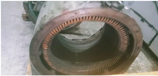
Fig 2.5. Stator construction of 3p-SR-IM - Source: forumautomation.com and photograph
