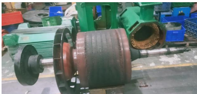
Figure 2. 5: Photograph of Rotor construction of the studied 3p-SR-IM - Farhan Mahaputra Rahman (20-06-2022) [PT. REMS]
