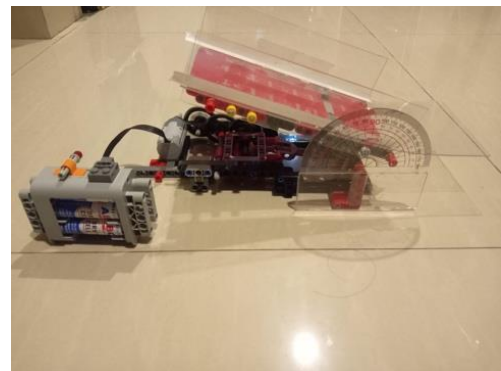
Figure 1. Lego structured equipment to measure angle of repose
