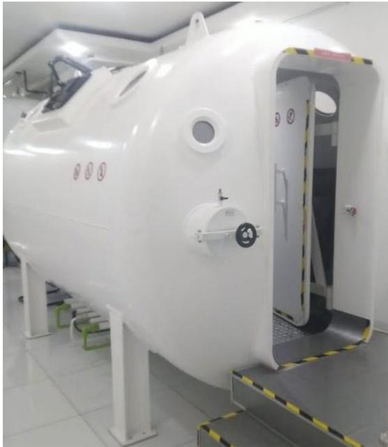
Picture 1. A picture of Multiplace chamber in Asyifa Remopa Hyperbaric Clinic. The chamber is made of stainless steel and the glass use PMMA, Picture by Roderick Osman Chandra
